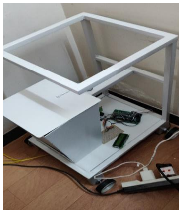
Fig 3: Motor drive and Sensors integrated in the dustbin
